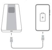
Charging capabilities of the USB Type-C port: Charging the Mobile WiFi: 10 V/2.25 A (MAX)/9 V/2 A (MAX) for fast charging and 5 V/2 A for other charging modes.
